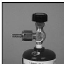
Figure 5. Installation without regulator, but with hose-barb adapter, for noncorrosive, liquefied gases packaged in low pressure flat-bottom cylinders.
